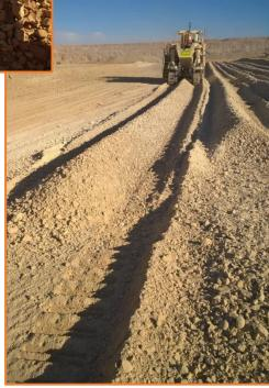
Between December 2015 and January 2016 Global Civil and Mining (GCM) carried out a surface mining trial at Olympic dam employing a Wirtgen 2500 Surface Miner (2500SM) in windrow mode.
